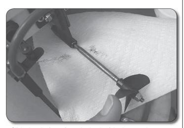
3. Slide the shaft out from the back of the boat and re-grease. Reinstall and retighten the cable.
