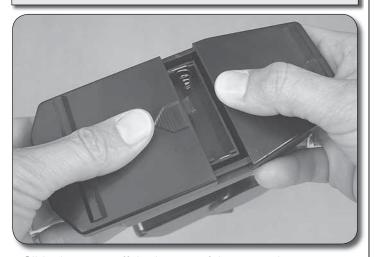
1. Slide the cover off the bottom of the transmitter.
