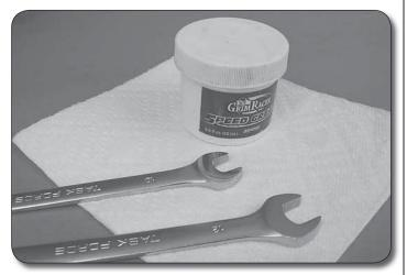
1. You are going to need one 10mm open end wrench and one 12mm open end wrench and some grease.
